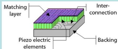
The 2D probe is developed by Vernon, Tours. It consists of 32 by 32 elements, sized 0.4 mm squared. The first prototype is ready and ErasmusMC (Rotterdam) is currently measuring the impedance and pulse echo response.
